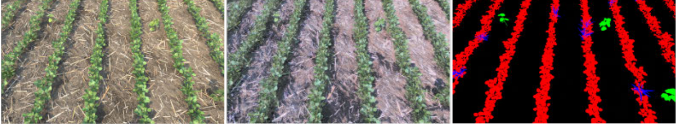
Figure 4. An example image from our synthetic dataset: (left) rendered, (middle) domain adapted, (right) generated labels, where red is crop, green is broadleaf weed, and blue is grassy weed.
