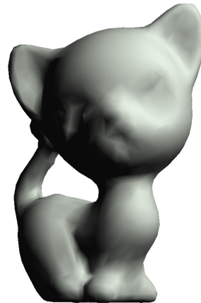
Figure 5.4: The effect of rendering with vertex normals. (a) The mesh has been rendered with flat faces; (b) the mesh has been rendered with vertex normals computed by Algorithm 5.1.
