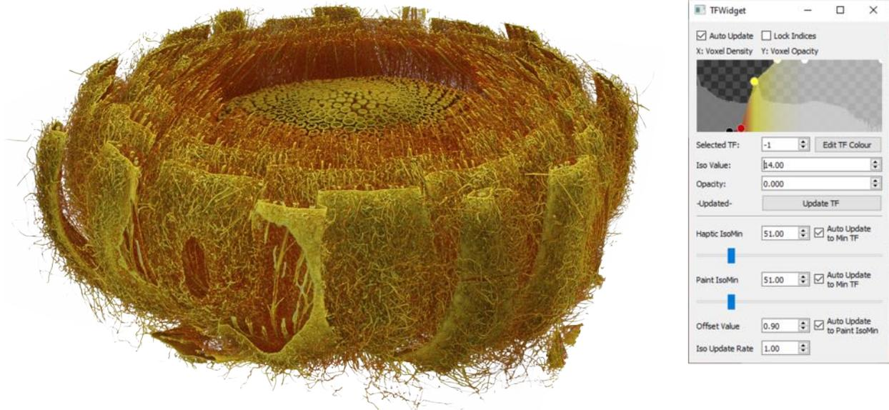
Figure 4.6: (left) The volume coloured by a transfer function. (right) The transfer function widget consists of a histogram of all intensity values within volumetric data, editable control points, and lines that interpolate the colour and opacity in between each successive control point.
