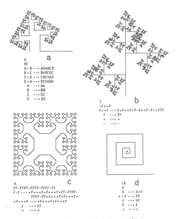
Fig. 4. Examples of pictures obtained using generalized L-systems. In these examples the set of productions is ordered. If more than one production can be applied, the production higher in the list is chosen.
