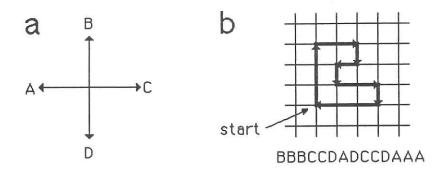
Fig. 1. (a) Assignment of letters to line segments in chain coding. (b) The chain representation of an example picture.
