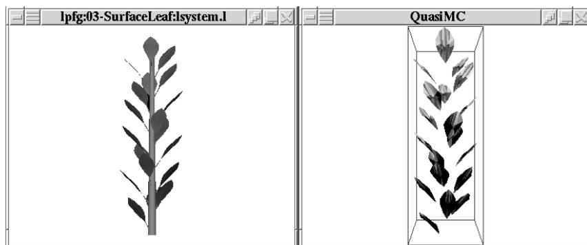
Figure 1: The plant-light simulation software from the user's perspective: on the left, the plant simulator *lpfg*, and on the right, the light environment simulator *QuasiMC*. The *QuasiMC* program shows the plant organs which are included in the light distribution simulation.
