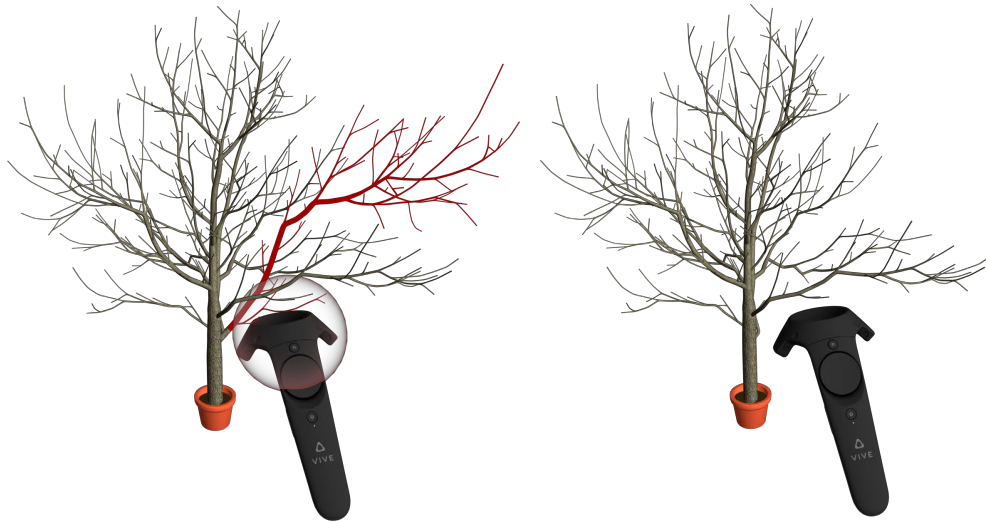
Figure 11.2: Pruning of a branch on the tree. A partial press of the trigger previews nodes that would be pruned, while a full press removes them.
