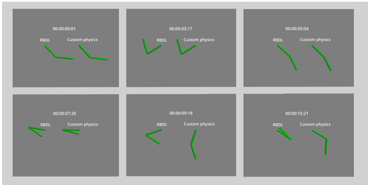
Figure 8.4: Two double physical pendulums side by side. Notice the chaotic motion starting at the 4th frame.
