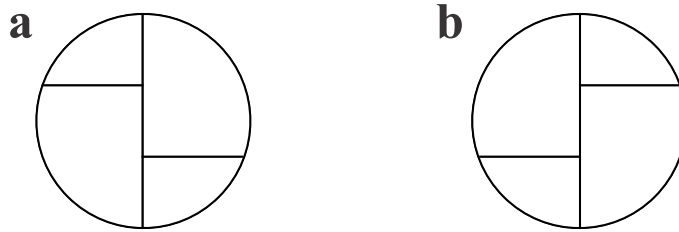
Figure 7.4: Offsets between four regions that result from the division of two regions sharing a common edge: (a) Z-offset, (b) S-offset
