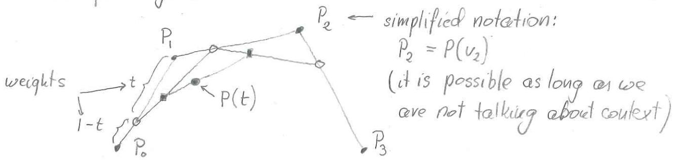
Like subdivision algorithms (including the "chasing game"), the de Casteljau algorithm is a geometric construction. Unlike the subdivision algorithms, however, it returns only a single point for a given value of parameter  $t$  (the entire curve is obtained by sweeping  $t$  from 0 to 1).
